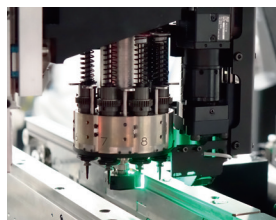
Component side recognition camera
